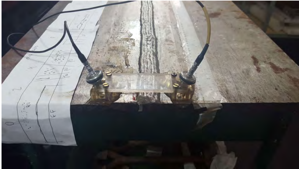
Figure 4.5: Specimen and ToFD ultrasonic probes.
