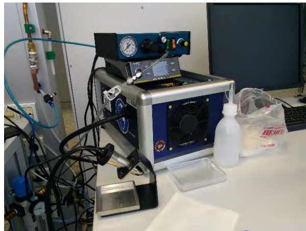
Figure A.7: Semi-Automatic Dispenser
