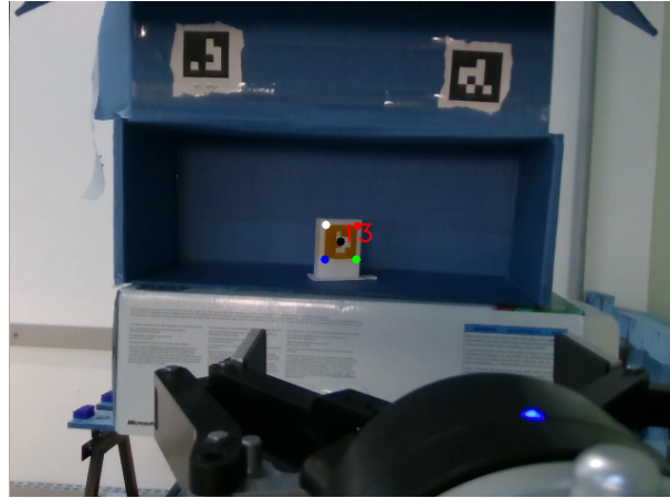
Figure 4.31: Experiment 1.1.2: Tag Detection while rotated 15 degrees on the Y axis.
