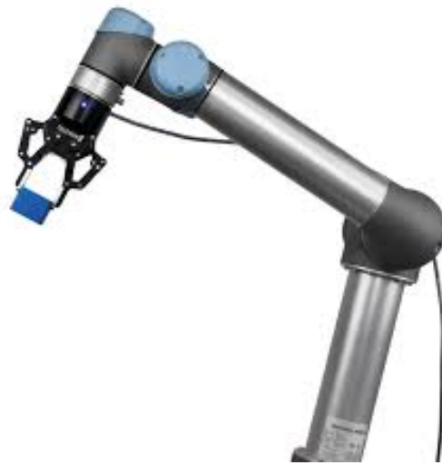
Figure 3.1: UR5 with Robotiq Gripper. Source: Universal Robots.
