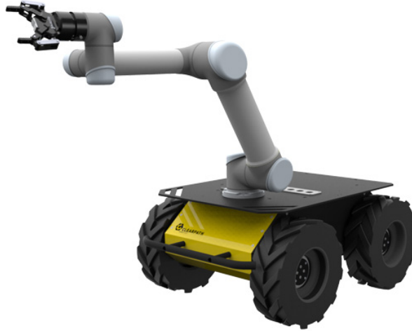
Figure 4.65: UR5 mounted on Husky. Source: Clearpath.
