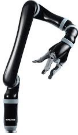
Figure 3.2: JACO robotic arm. Source: Kinova Robots.
