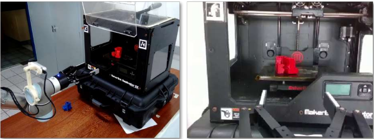
Figure 1.2: Additive Manufacturing Unit for 6D grasping testing.
