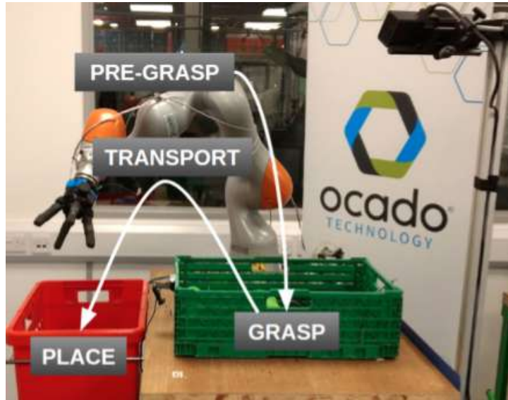
Figure 2.16: Phases considered for benchmarking in pick-and-place tasks (MNYUSIWALLA et al., 2020).
