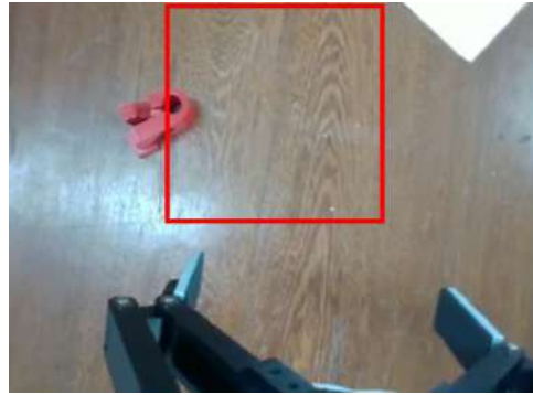
Figure 3.2: Using the GG-CNN, a grasp is not generated for objects outside the GG-CNN area (red box).
